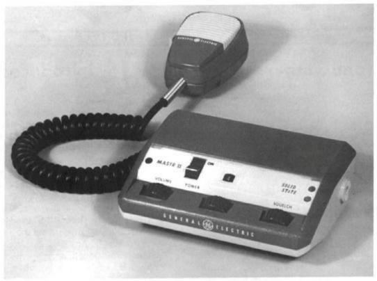
The MASTR II incorporates more of the latest in monolithic and hybrid circuitry, ceramic capacitors, silicon transistors and monolithic crystal filters than any contemporary design. Engineered to serve the toughest communications assignments, it offers the user the highest dependability in the industry in every kind of weather, under every conceivable condition of stress. The design approach takes into consideration the real life environment in which some two-way radios are required to operate.
