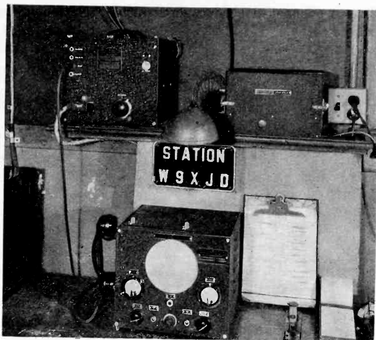
Fig. 16—Fifteen-watt 30- to 42-megacycle transmitter and superheterodyne-superregenerative receiver working from a common power supply and on a single antenna installed in Whiting, Indiana.
