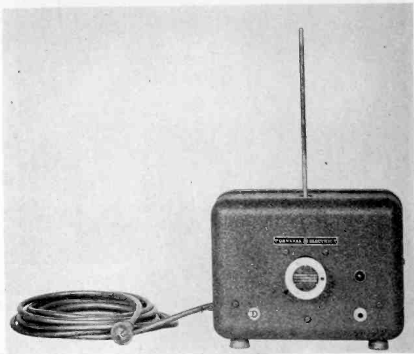
Fig. 14—Crystal controlled frequency monitor, 30 to 42 megacycles, for checking frequency settings.
