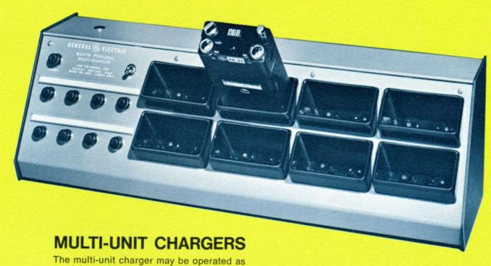
The multi-unit charger may be operated as an eight-position charger, or two slave units may be connected to a master giving a total of 24 charging positions. Each position is equipped with an indicator lamp and an automatic trickle switch. All multi-chargers may be either desk or wall mounted.
