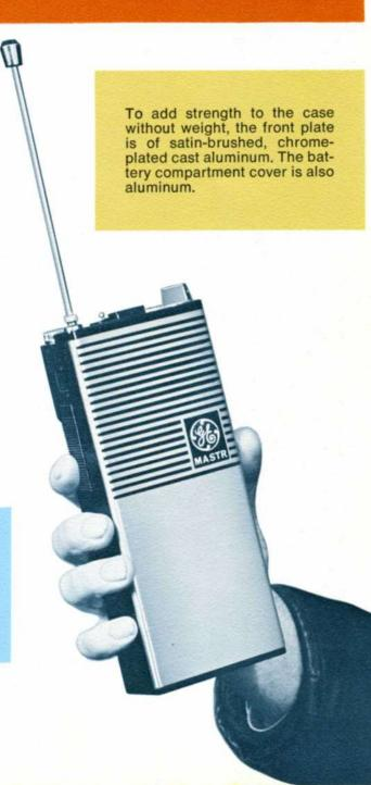
All controls except the push-to-talk switch and the high-low power switch are mounted on the top surface of the unit.
