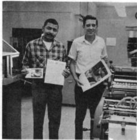
THE NEWS IS PREPARED FOR PRINTING... Photographic Dark Room Operator St. Clair Anderson (left) shows photo and "dummy" of front page from which he will shoot negatives, and Offset Operator Ray Reynolds shows negative which will be used to "burn" a plate to be run on the press at right. The entire operation in Reproduction must be done in a minimum of time to permit distribution prior to employees' lunch hour.
