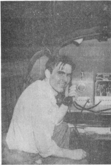
THIS PHOTO OF JOHN (taken during the early 1940's) shows how power supply units for mobile radio equipment completely filled the truck of an automobile.
