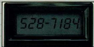
Backlit LCD display for easy viewing night and day.
