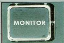
Monitor switch lets you check on radio traffic without coming off-hook.
