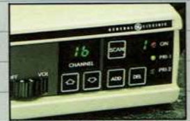
Optional multi-channel scan with dual priority feature assures important calls are not missed.
