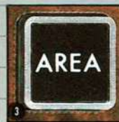
Area switch allows roaming or wide area service.
