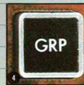
Group switch allows selective calling of five different groups or fleets, each with privacy.
