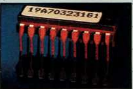
Electrically Erasable Programmable Memory allows fast reconfiguration of Delta-S radio systems in the field — with no need to remove the covers.
